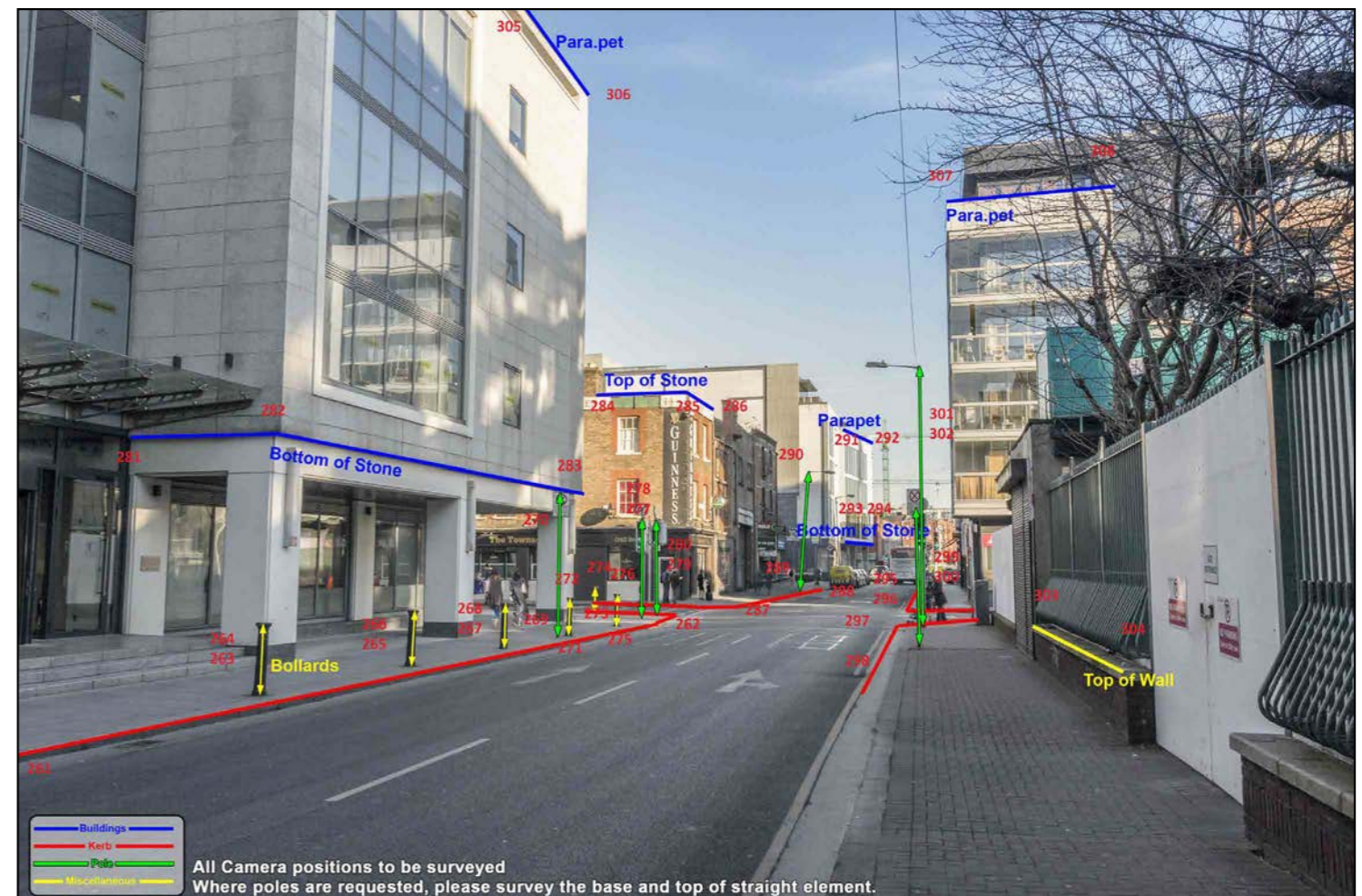
Fig.8: Fixed reference points fully surveyed and numbered.
